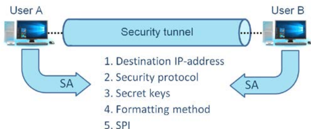
Fig. 4.3. Between two ending points of VPN logical connection which in standards of IPSec wears the name "Secure Association" is set
